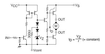
As shown in the above diagram, the V cont pin outputs the voltage of the band gap Zener V<sub>Z</sub> + V<sub>F</sub> (=1.93V). In normal use, this pin is left open.
